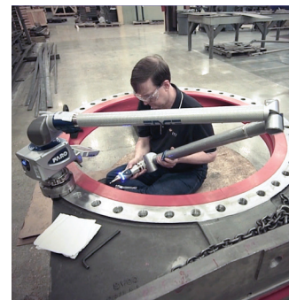
Large Urethane Lined Valve being measured with CMM arm.
