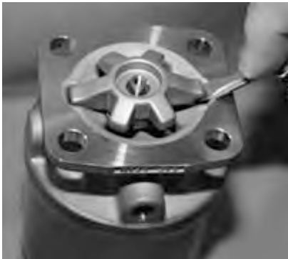
Figure 6: Remove the compressor
