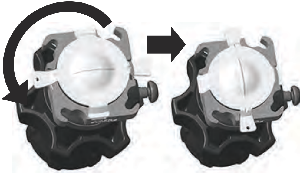
Figure 27: Installation de la membrane
