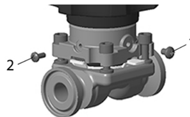
Figure 11: BioviZion/PFuZion 0.5 inch with sealed bonnet screw and pressure ring retention
