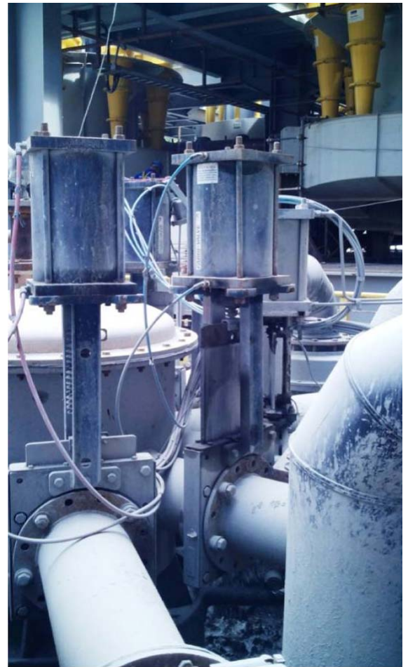
Valve is used for isolation of hydroclones that classify or separate particles present in nickel slurry
