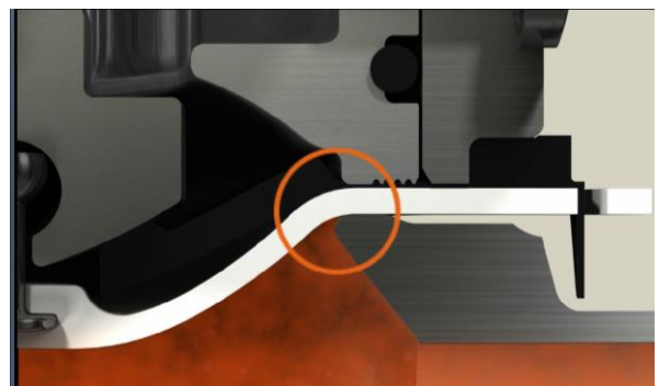
Active Thermal Compensation system assures contamination free shell seal
