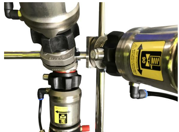
Seal issues were eliminated after the 36 EnviZion valves were installed
